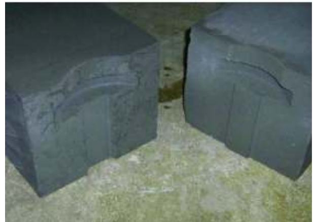
“Jumbo” Aircrete blocks with tongue and groove features and hand grips (image, BRE Information Paper IP 7/05)
