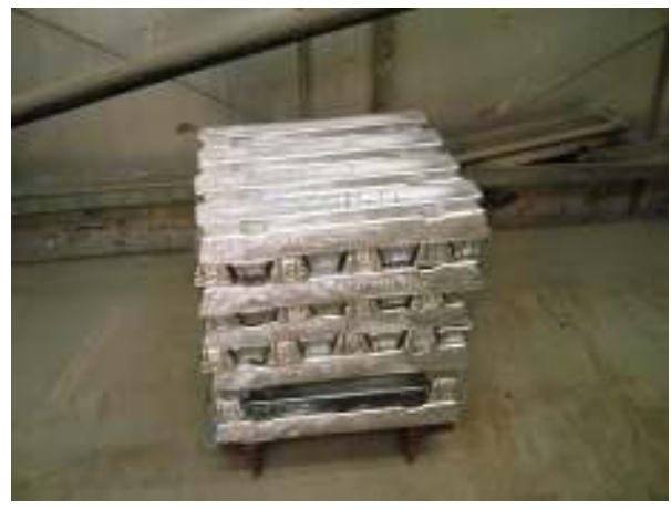
Figure 7: Aluminium ingots from aluminium dross recycling
