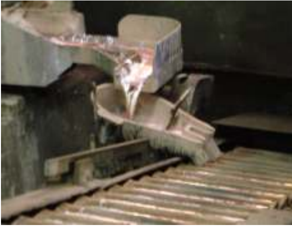
Figure 6: The casting process of metal aluminium produced from dross reprocessing
