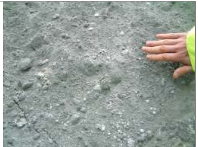
Figure 2: White dross with low aluminium content
