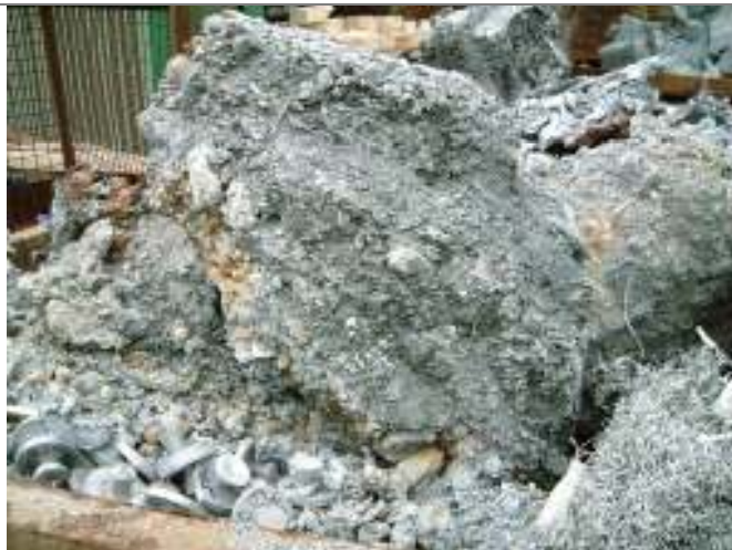
Figure 1: White dross in lump form with high aluminium content
