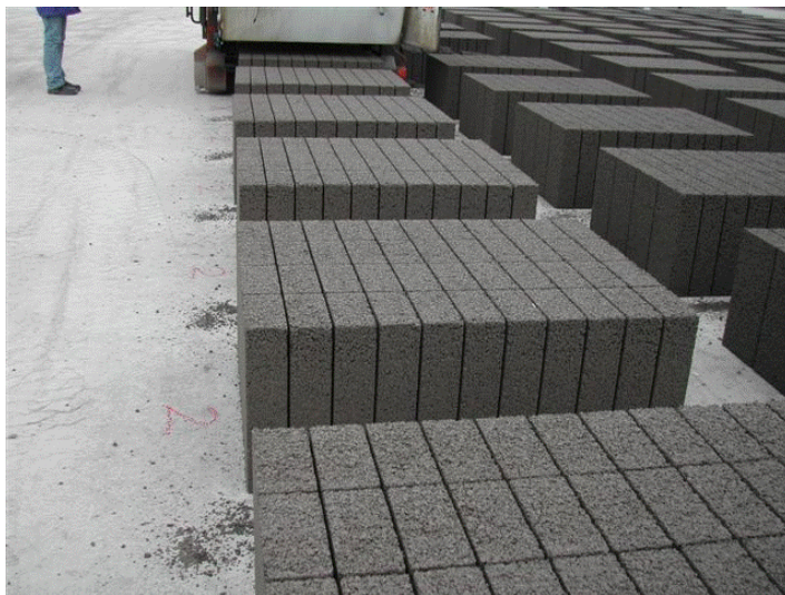
Figure 3: Typical dense aggregate concrete building blocks in the factory (Stowell Concrete)
