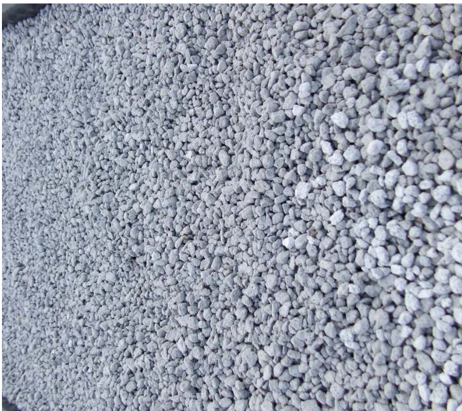
Figure 2: Aircrete as being used for test as a green roof substrate, sometimes with organic matter added
