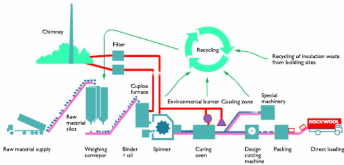
Figure 1: Schematic of the manufacture of mineral wool (source Rockwool® website)
