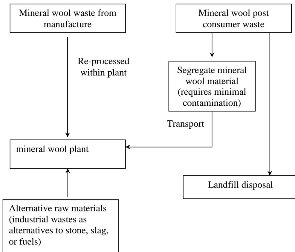
Figure 4: Alternative resources for mineral wool manufacture
