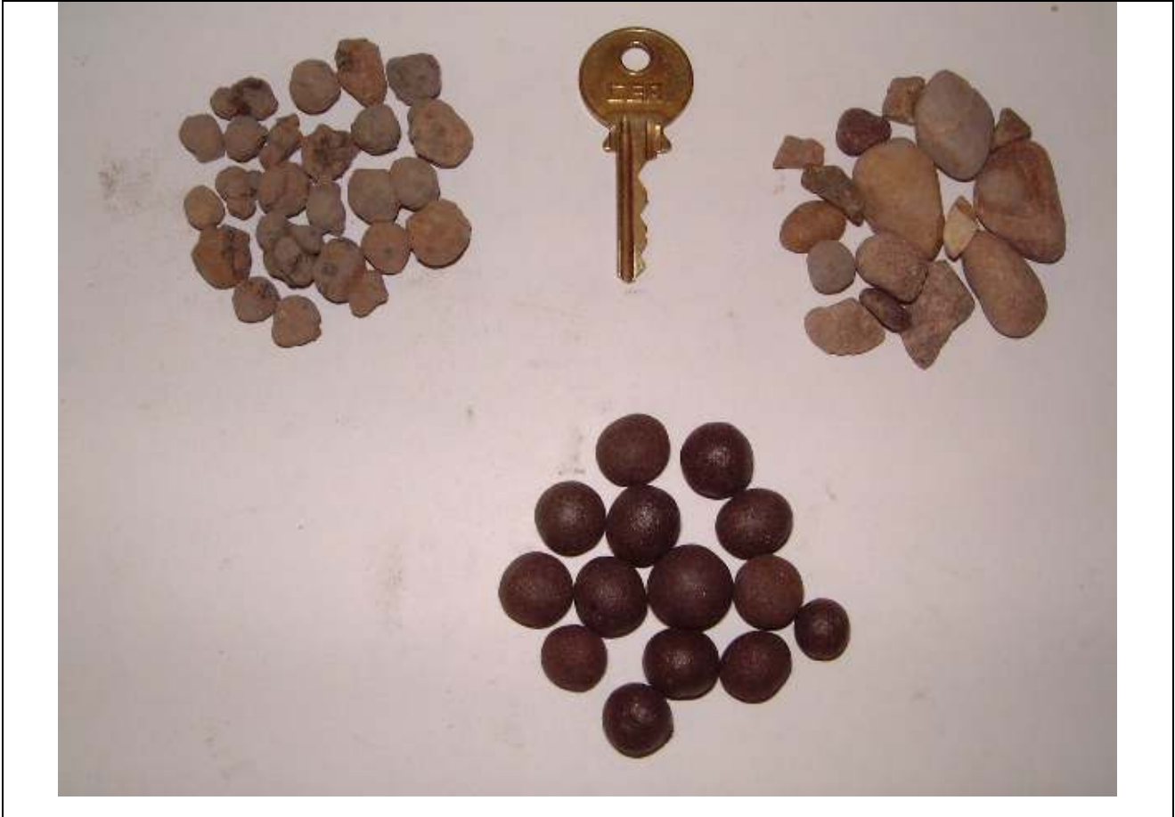
Figure 4: Photograph of aggregate made from granite filter cake washings (bottom) lytag (left) and natural gravel (right)
